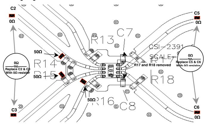
SY89208V DC-Coupled Loading Diagram
